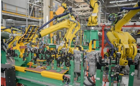
Automated robotized production line designed and implemented by SEGULA Technologies for a European automotive customer (©SEGULA Technologies)
